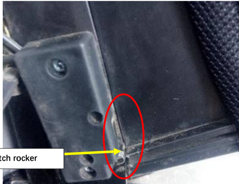
Fig.14-2 Switch rocker- Closed state
