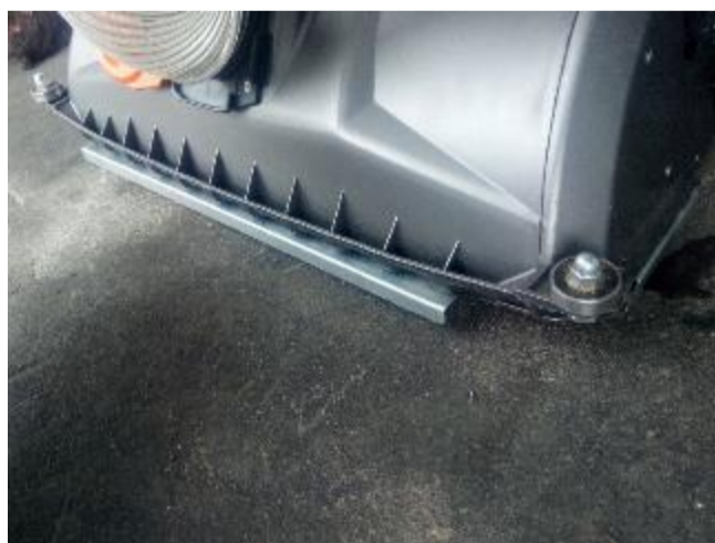
Fig.30-2 The baffle is inserted into place
