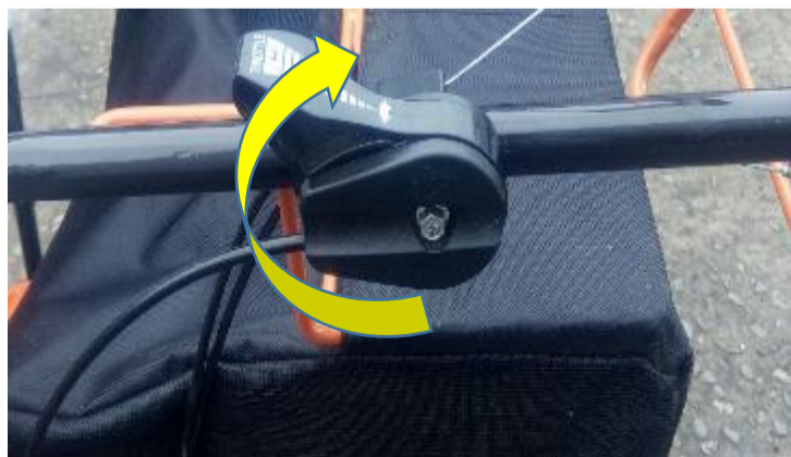
Fig.18-1 Throttle handle- Engine startup state
