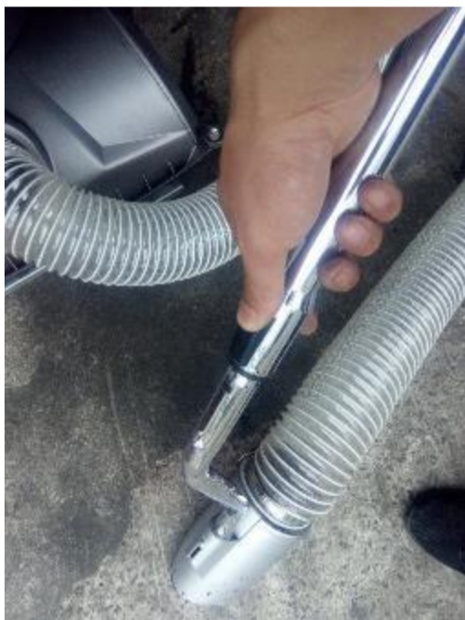
Fig.32-1 Push open the lock
