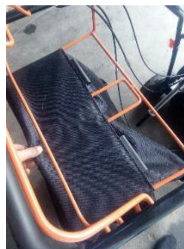
Fig.37-3 Remove the collection bag
