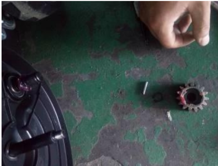
Fig.39-2 Add grease to the output shaft
