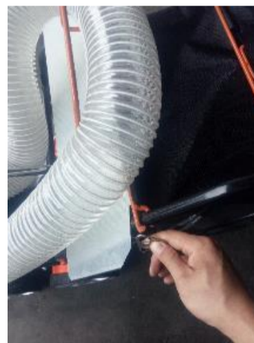
Fig.37-2 Remove the collection bag hanging plate
