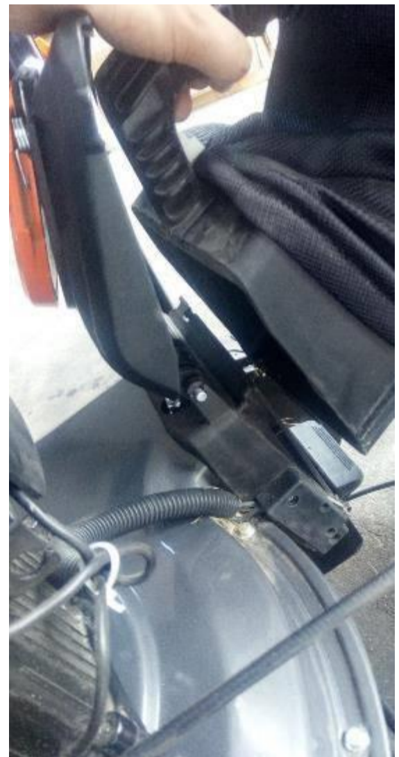
Fig.10-6 Insert back cover bracket
